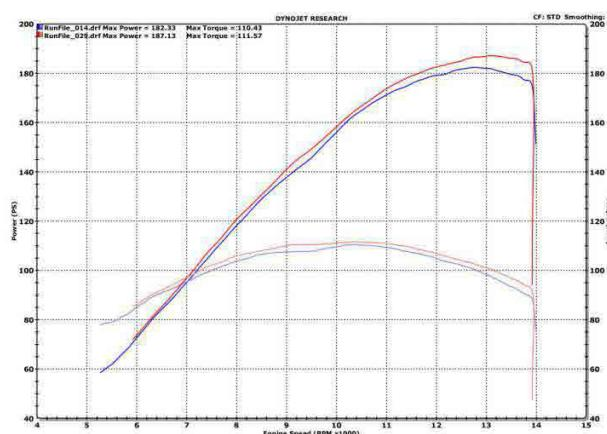
RunFile\_014.drf - 13/11/2014 13:56:29 Run Type: RO Run Conditions: 24.08 °C, 1000.29 mBars, Humidity: 33%, STD: 1.02
