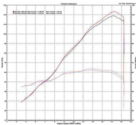
RunFile\_005.dat - 20/01/2015 19:46:50 Run Type: RO Run Conditions: 16.94 °C, 1000.03 mBar, Humidity: 35%, DIN: 1.01 GROOVE HRDLA
